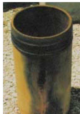
Cavitation and liner perforation
