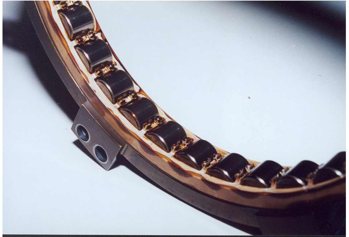
View of N°6 HPT bearing at overhaul, 24,000 h with TN 600
