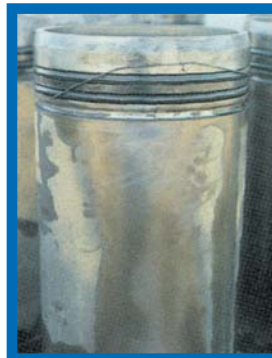
After 14,400 hours with NORKOOL coolant – no cylinder liner cavitation corrosion
