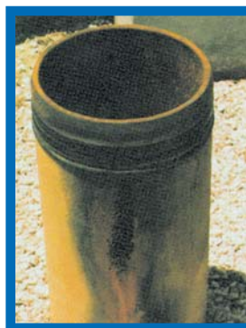
After 5,500 hours without NORKOOL coolant – cavitation and liner perforation
